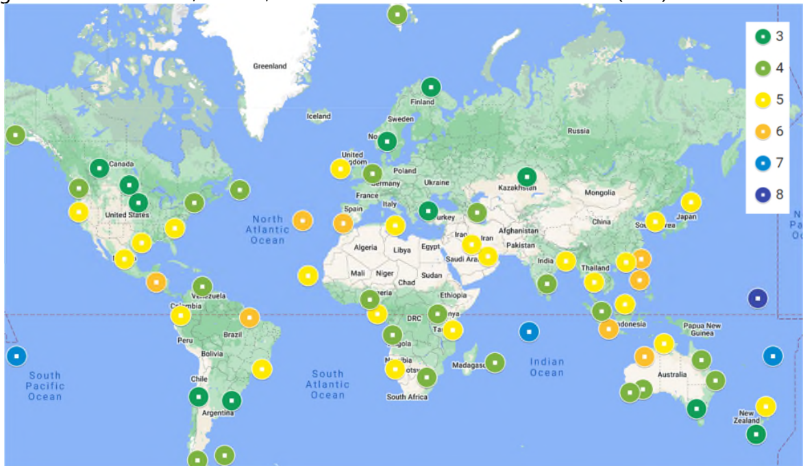
Figure 2: G4+ 95% height accuracy in centimetre. (Results may differ depending on receiver type.)
